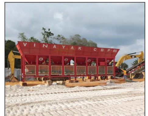
INCLINE STORAGE BIN
